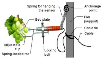
A stationary pier (support) is to be used for positioning the sensor and its cable. At first, adjust the sensor's clip to the fruit diameter by using a step scale located on the sensor's body.
