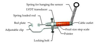
Standard cable length between sensor and signal conditioner is 0.5 meter. The standard output cable length is 3.5 m (4 m total length). The length may be customized in the order if need be.
