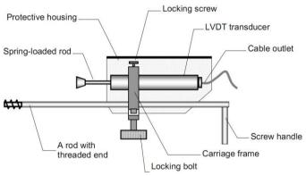
The probe is connected by a standard 0.5-meter cable to the waterproof tube with the signal conditioner inside. A signal conditioner provides excitation of the LVDT and production of standard linear output signal.
