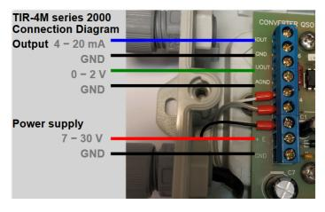
First, please choose a right output cable for connecting the sensor to a datalogger. The cable must be round with four wires. The maximal diameter of the cable is 6.5 mm. The cable length shall not exceed 10 m for 0 to 2 Vdc output and with about 1 km maximal length for 4 to 20 mA.
