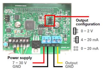
First, please choose a right output cable for connecting the sensor to a datalogger. The cable must be round with four wires. The maximal diameter of the cable is 6.5 mm. The cable length shall not exceed 10 m for 0 to 2 Vdc output (model SD-xM) and with about 1 km maximal length for 4 to 20 mA or 0 to 20 mA output (model SD-xMi).
