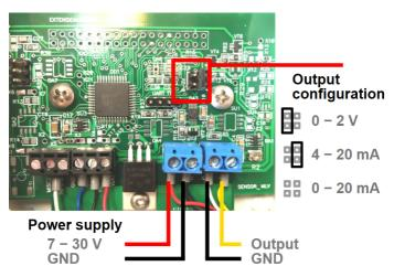
First, please choose a right output cable for connecting the sensor to a datalogger. The cable must be round with four wires. The maximal diameter of the cable is 6.5 mm. The cable length shall not exceed 10 m for 0 to 2 Vdc output (model LT-xM) and with about 1 km maximal length for 4 to 20 mA or 0 to 20 mA output (model LT-xMi).
