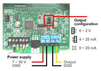
First, please choose a right output cable for connecting the sensor to a datalogger. The cable must be round with four wires. The maximal diameter of the cable is 6.5 mm. The cable length shall not exceed 10 m for 0 to 2 Vdc output (model Fl-xM) and with about 1 km maximal length for 4 to 20 mA or 0 to 20 mA output (model Fl-xMi).
