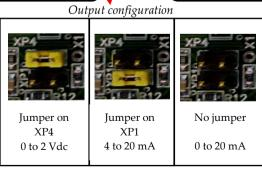
Maximal length of the output cable is 4 m for sensors with voltage output and up to 200 m for sensors with 4 to 20 and 0 to 20 mA output.
