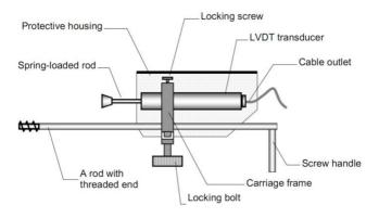
The probe is connected by a standard 1-meter cable to the waterproof box with the signal conditioner inside. A signal conditioner provides excitation of the LVDT and production of standard linear output signal.
