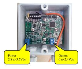
Maximal length of the output cable is 10 m.
