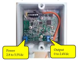
Maximal length of the output cable is 10 m.
