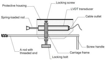
The probe is connected by a standard 2-meter cable to the waterproof box with the signal conditioner inside. A signal conditioner provides excitation of the LVDT and production of standard linear output signal. The output cable length should be specified in the order if required.
