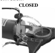
Correct orientation of the leaf chamber in the Northern hemisphere is shown in the picture below. In the Southern hemisphere, orientation must be opposite.
